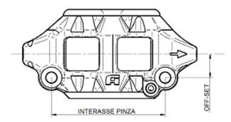
When choosing a brake caliper, always verify the compatibility between the "distance" and "Off-set" with the and the brake rotors of the motorcycle.
